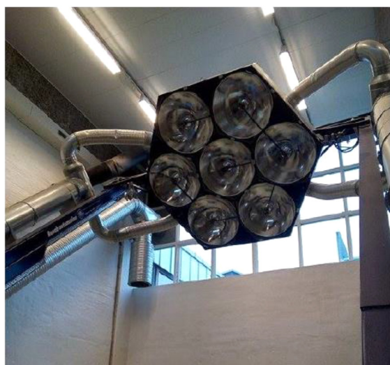
Fig. 12. Left: indoor solar simulator in laboratory. Right: level of irradiation on the leaning collector in laboratory. (colour)
